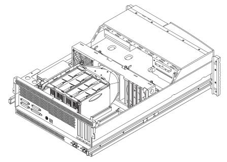
Figure 3. Sun Enterprise 420R server chassis with access panel removed, provides full access to internal options
