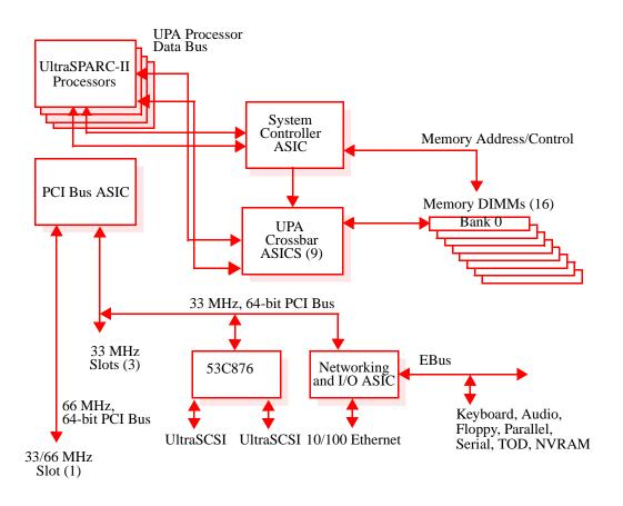
Figure 2. Architecture of the Sun Enterprise 420R server system
