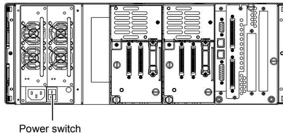
Figure 30 Power Switches, L100
