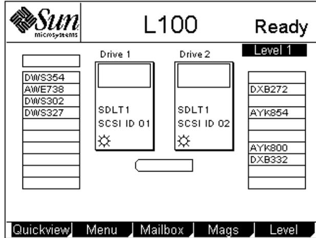
At the bottom of each GUI screen are up to five button labels. These labels indicate the functions of the five push buttons below the GUI. To select a function, press the push button directly below the button label on the GUI screen (see [figure 33](#)).
