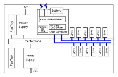
Figure 3. Sun StorEdge A1000 system architecture
