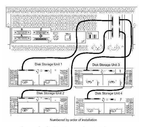
Figure 2. Sun StorEdge N8200 configured with four arrays
