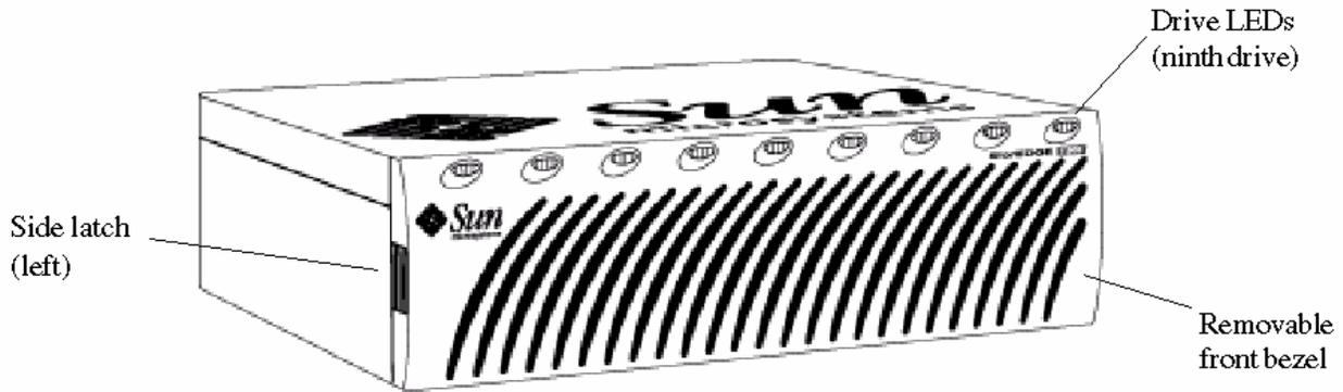
**Figure 5.** Front view of the Sun StorEdge T3 controller unit
