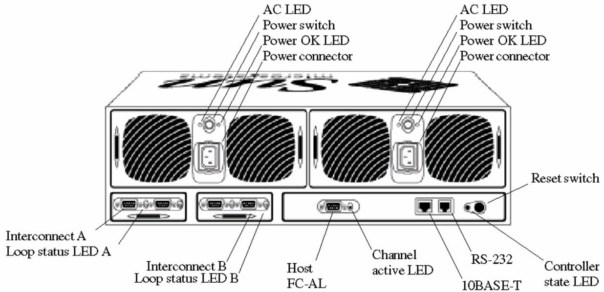
Figure 6. Rear view of the Sun StorEdge T3 controller unit
