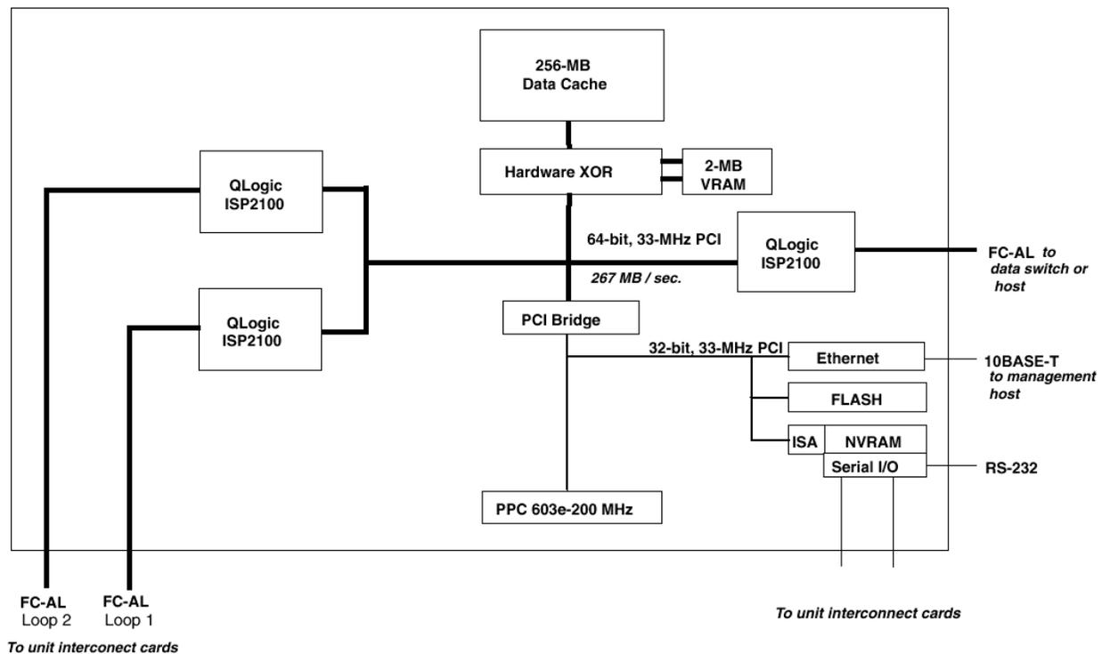
**Figure 4.** Controller architecture
