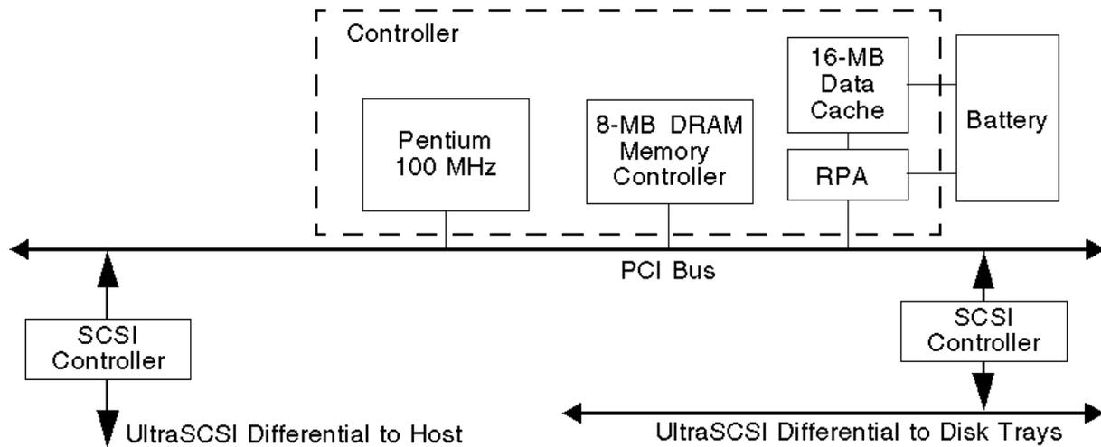
Figure 4. Sun StorEdge A1000 array controller board architecture
