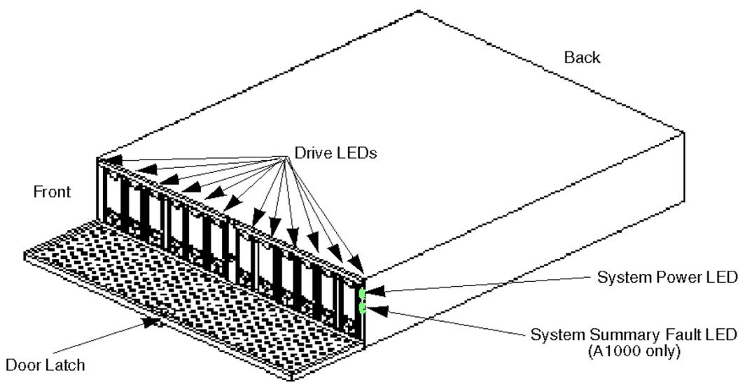
Figure 6. Sun StorEdge A1000 and D1000 arrays front view
