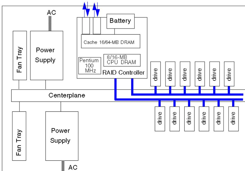
Figure 2. Sun StorEdge A1000 array system architecture
