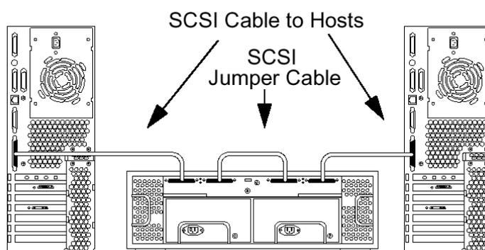
**Figure 13.** Bridged Sun StorEdge D1000 array connected to dual hosts
