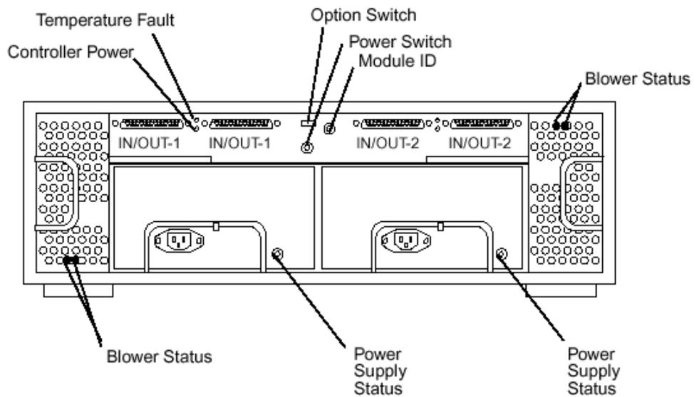
Figure 8. Sun StorEdge D1000 array rear view
