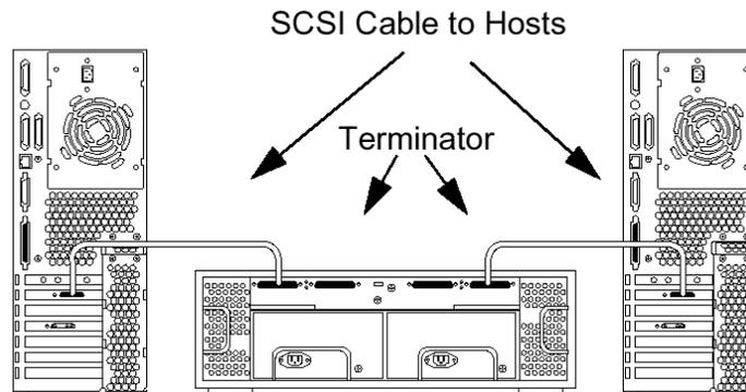
Figure 12. Unbridged Sun StorEdge D1000 array connected to two hosts
