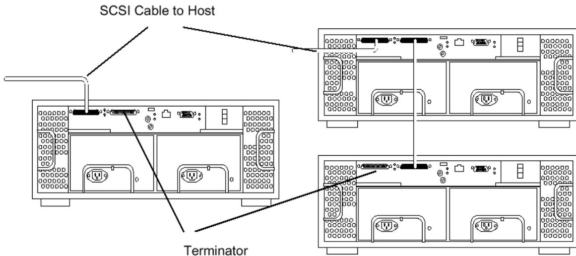
Figure 9. Single and Daisy-chained Sun StorEdge A1000 array connected to a single host
