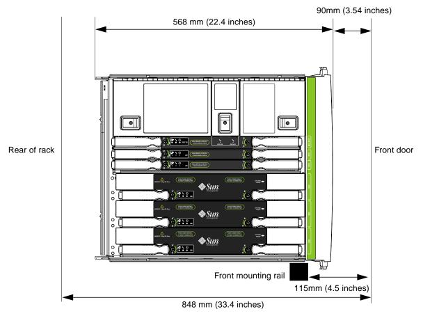
FIGURE 4-4 Maximum Rack Depth Requirement
