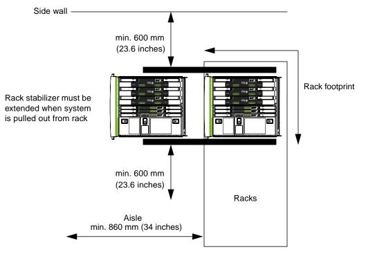
FIGURE 4-5 Service Access – Floor Space (plan view)
