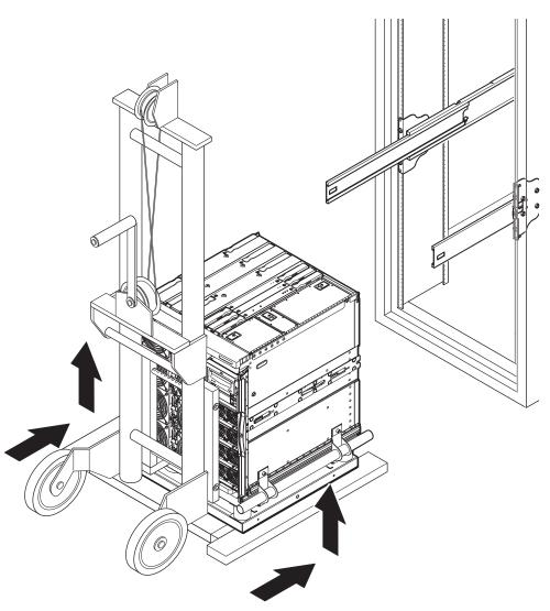
$\ensuremath{\mathsf{FIGURE}}\xspace$  5-10 Raising the System Prior to Insertion in the Rack
