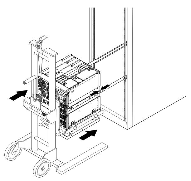
$\ensuremath{\mathsf{FIGURE}}\xspace$  5-11 Aligning the System with the Rackmount Slides
