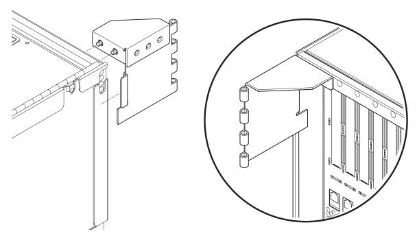
FIGURE 5-18 Fitting the Upper Pivot Bracket
