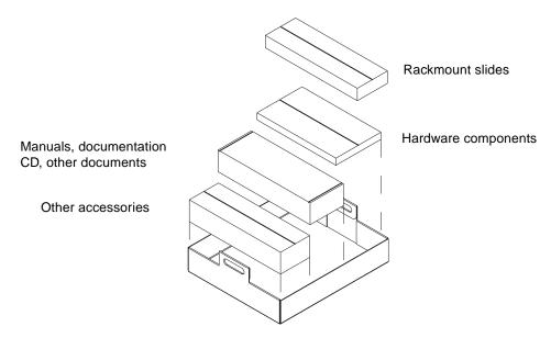
FIGURE 5-2 Unpacking the System #2 – Shipkit Tray
