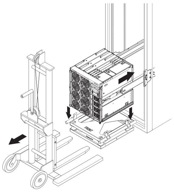
FIGURE 5-12 Engaging the Rackmount Slides and Glides
