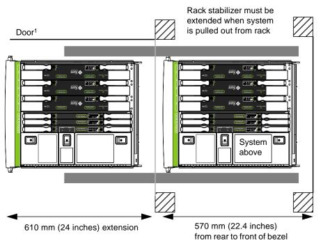
FIGURE 4-7 Service Access – Cabinet (plan view)
