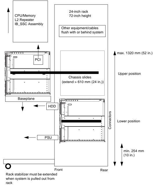
FIGURE 4-6 Service Access (side view)
