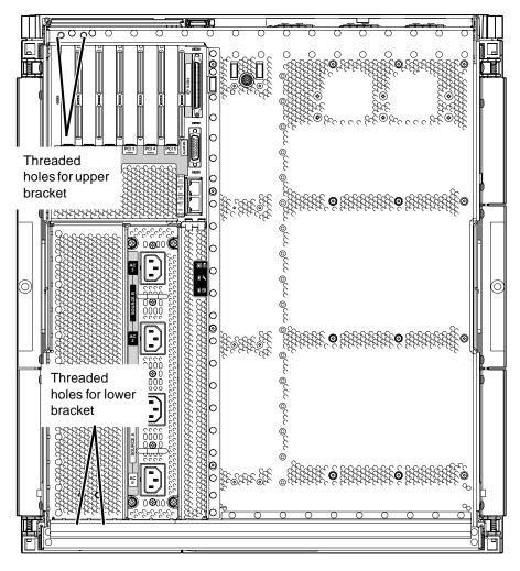
FIGURE 5-15 Locations of Pivot Bracket Mounting Holes
