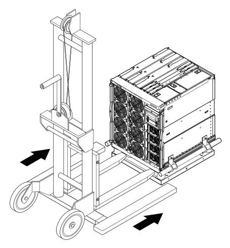
FIGURE 5-5 Inserting the Lifting Device
