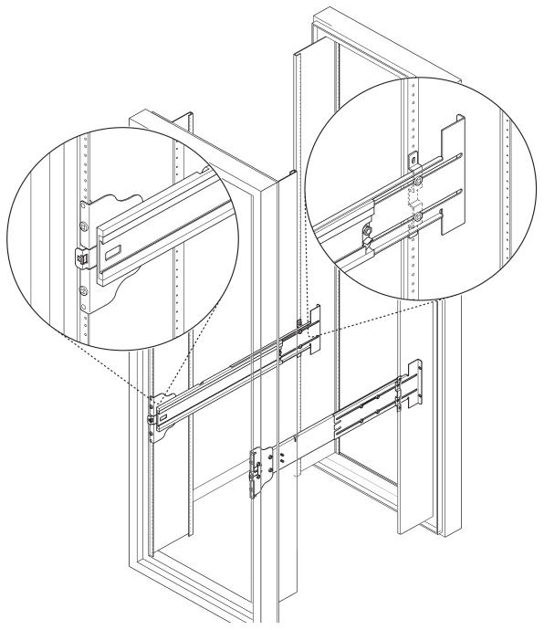
FIGURE 5-9 Installing Rackmounts in a Sun Rack
