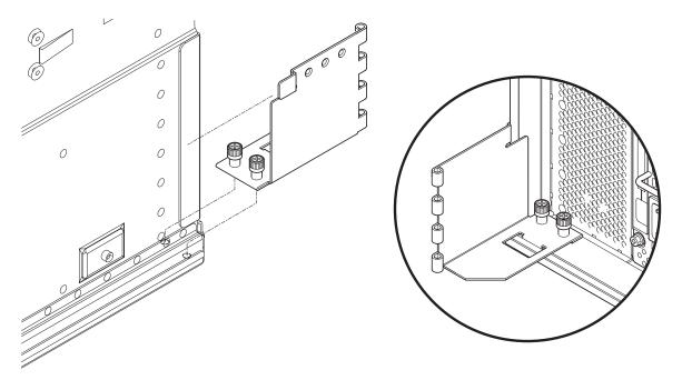
FIGURE 5-17 Fitting the Lower Pivot Bracket
