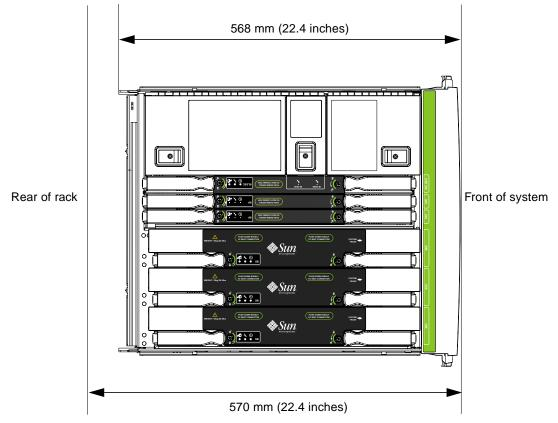
FIGURE 4-2 Minimum Rack Depth Requirement
