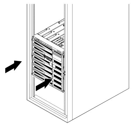
FIGURE 5-14 System Installed and Bezel Doors Reattached
