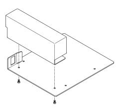
FIGURE B-2 Dismantling the Tape Drive Filler Panel
