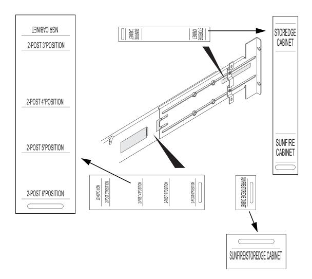
FIGURE 5-8 Rackmount Positioning Guidance Labels
