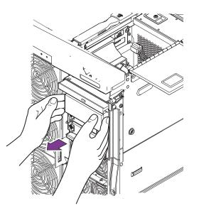
FIGURE B-6 Pulling Out the Media Bay a Short Distance
