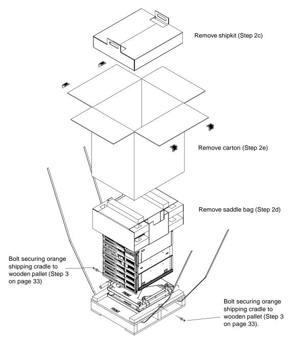
FIGURE 5-3 Unpacking the System #3 – Steps 2c, 2d, 2e and 2f
