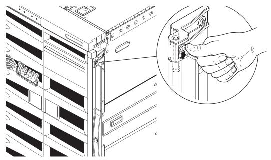
FIGURE 5-4 Bezel Hinge Release Mechanism
