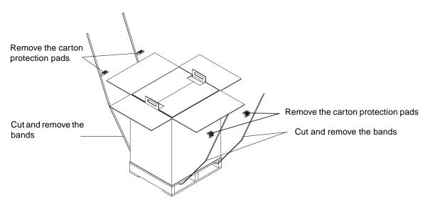
FIGURE 5-1 Unpacking the System – Opening the Carton – Steps 2a and 2b
