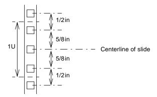
FIGURE 4-1 EIA/RETMA Universal Mounting Hole Pattern Dimensions
