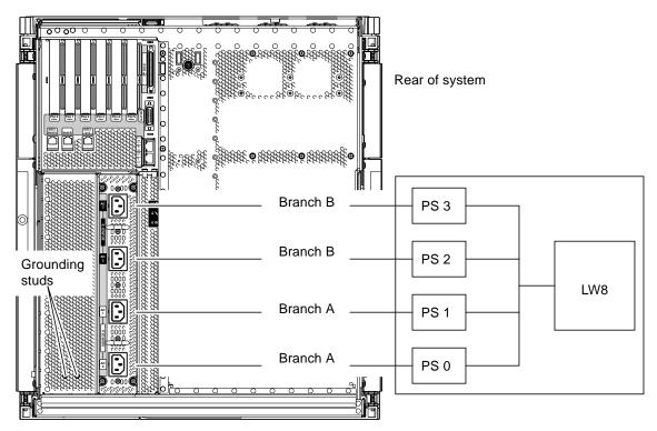
FIGURE 3-1 Connecting the Power Cords to Independent Branch Circuits for Optimum Redundancy
