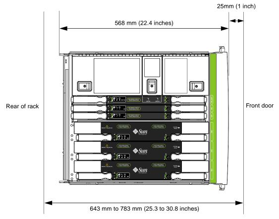
FIGURE 4-3 Typical Rack Depth Requirement
