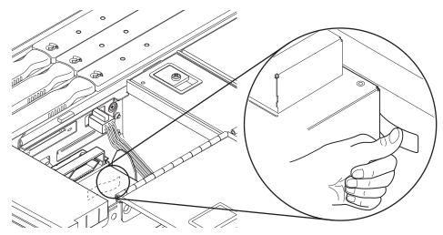
FIGURE B-5 Releasing the Media Bay Retaining Spring
