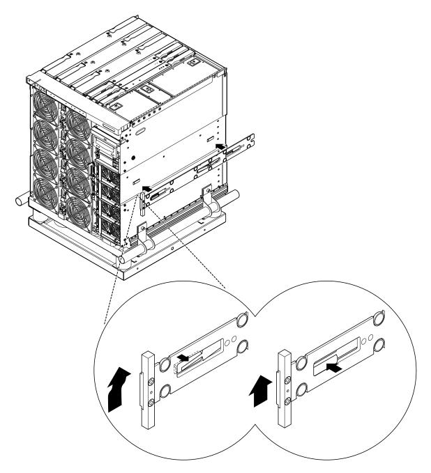
FIGURE 5-6 Installing the Rack Slides
