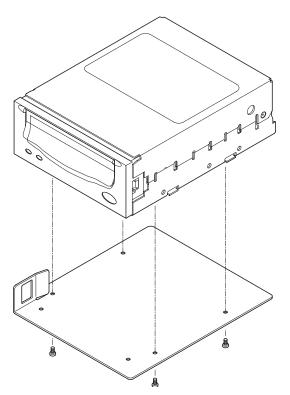
FIGURE B-3 Assembling the DAT Tape Drive
