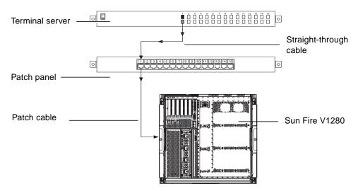
FIGURE C-1 Patch Panel Connection Between a Terminal Server and a Sun Fire V1280
