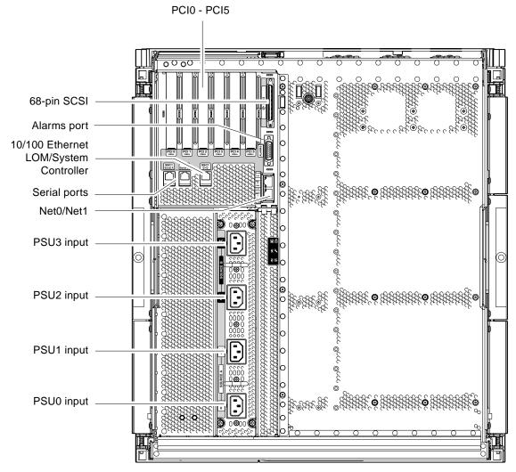
FIGURE A-1 External I/O Connections
