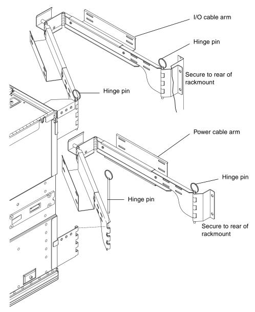
FIGURE 5-19 Assembling the Cable Arms
