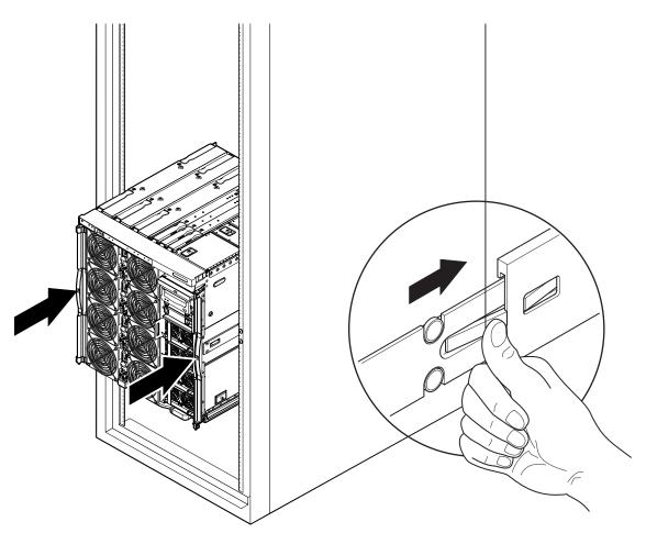
FIGURE 5-13 Pushing the System Fully into the Rack
