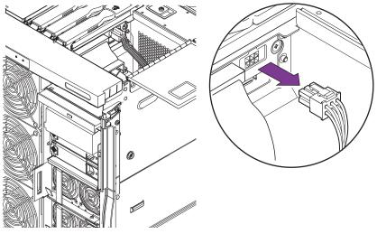
FIGURE B-4 Removing Cables from IB\_SSC Assembly to the Media Bay
