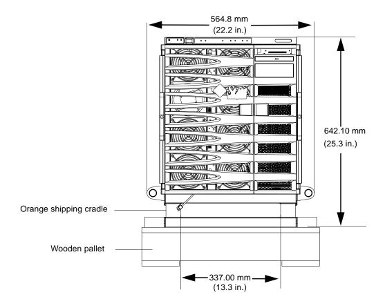
FIGURE 1-1 Dimensions – Front View
