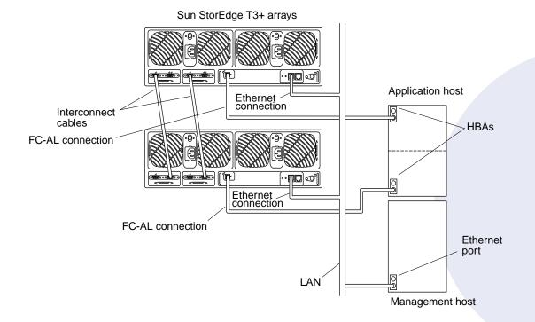
Connect the arrays to each other and to the hosts as shown in the diagram.
