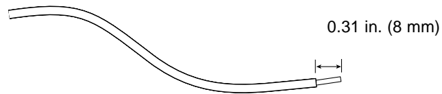
FIGURE 3-2 Stripping the Insulation From the Wire
