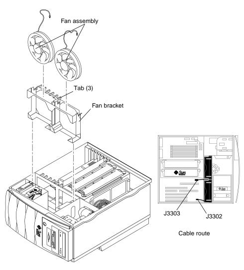
FIGURE 6-13 Removing and Replacing a Fan Assembly
