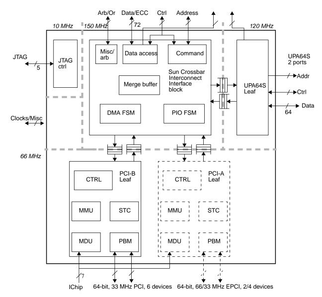
FIGURE C-6 SBC Block Diagram
