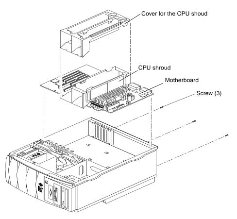
FIGURE 8-20 Removing and Replacing the Motherboard
