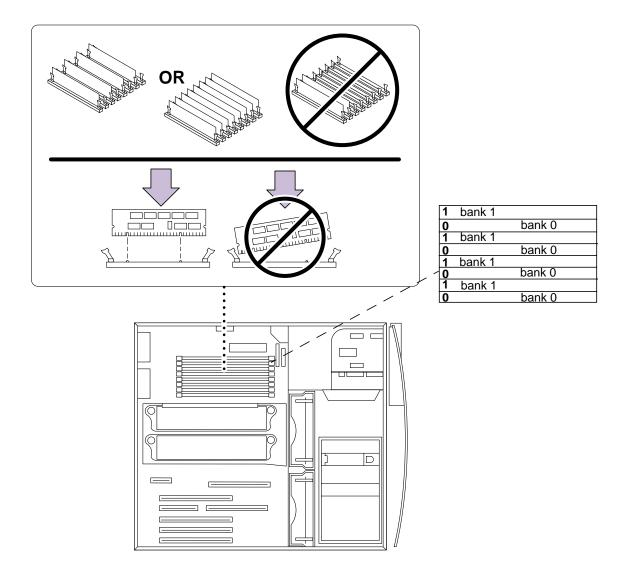
FIGURE 8-19 Removing and Replacing a DIMM
