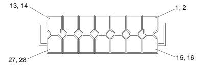
FIGURE B-2 Power Supply Connector J3601
