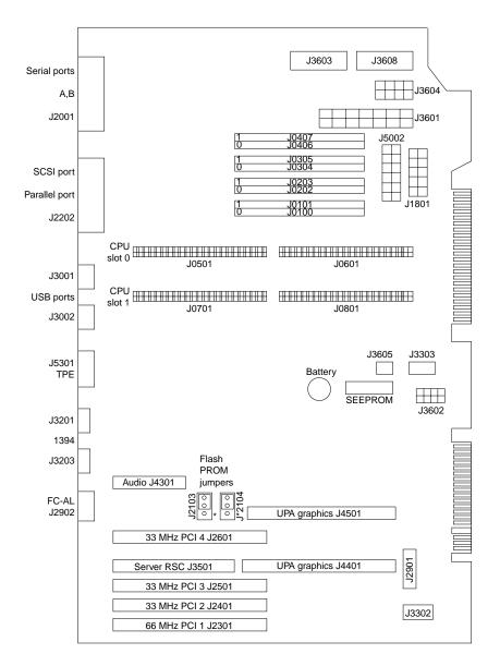
FIGURE 8-16 Graphics, EPCI, and PCI Card Slots
