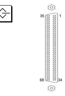
FIGURE B-8 UltraSCSI Connector Pin Configuration
