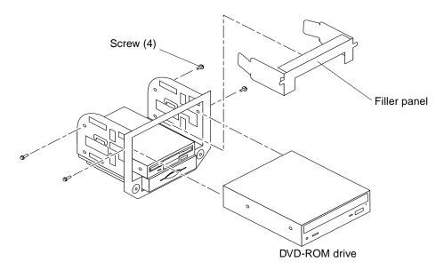
FIGURE 7-3 Removing and Replacing the DVD-ROM Drive
