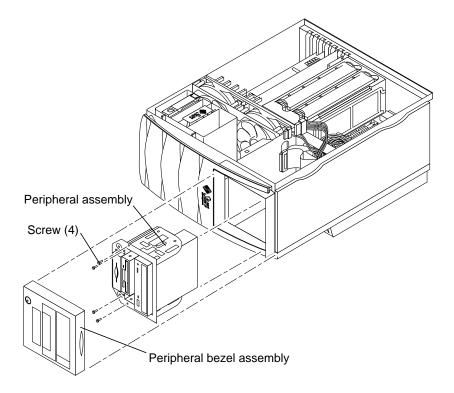
FIGURE 7-2 Removing and Replacing the Peripheral Assembly
