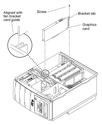
FIGURE 8-17 Removing and Replacing a Graphics Card
