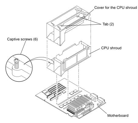
FIGURE 8-21 Removing and Replacing the CPU Shroud
