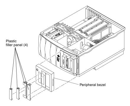
FIGURE 6-18 Removing and Replacing Plastic Filler Panels
