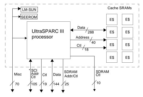
FIGURE C-2 UltraSPARC III Processor Functional Block Diagram
