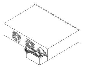
FIGURE 6-4 Dressing the Power Supply Cables
