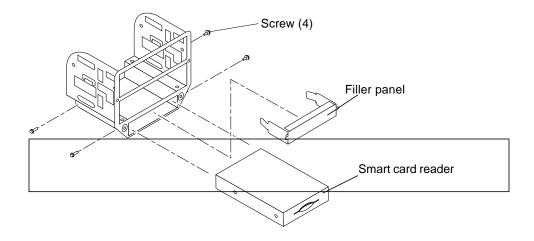
FIGURE 7-4 Removing and Replacing the Smart Card Reader
