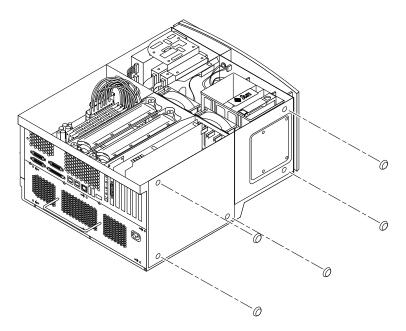
FIGURE 6-17 Removing and Replacing the Chassis Foot
