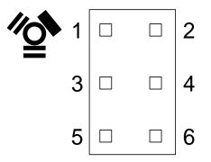
FIGURE B-11 IEEE 1394 Connector Pin Configuration
