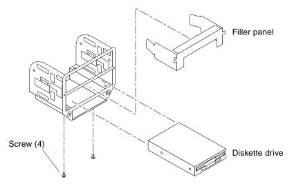
FIGURE 7-5 Removing and Replacing the Diskette Drive
