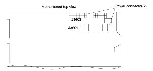
FIGURE 4-1 Power Supply Connector Jack Location
