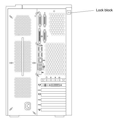
FIGURE 9-2 Lock Block Location
