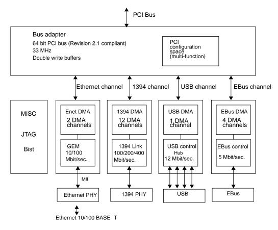
FIGURE C-7 PCIO-2 Block Diagram
