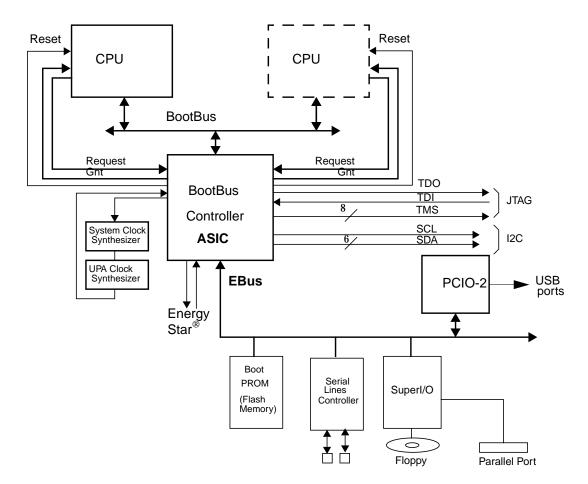
FIGURE C-9 Sun Blade 1000 and Sun Blade 2000 Boot Structure
