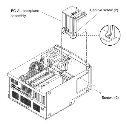
**8**. Disconnect the FC-AL backplane assembly from the chassis cutouts and lift it from the chassis.
