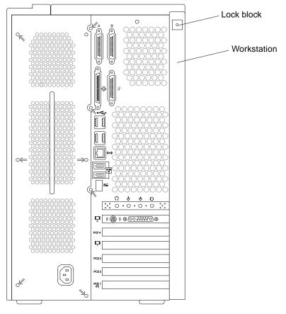
FIGURE 5-2 Lock Block Location
