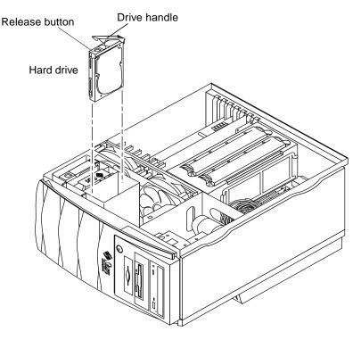
FIGURE 7-1 Removing and Replacing a Hard Drive
