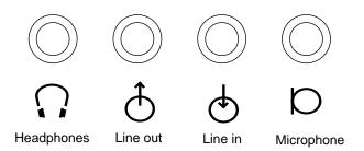
FIGURE B-13 Audio Connector Configuration
