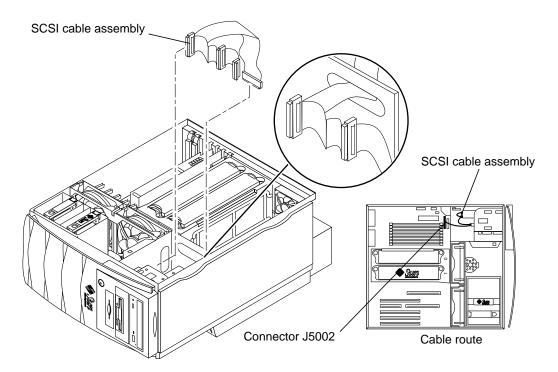
FIGURE 6-7 Removing and Replacing the SCSI Cable Assembly
