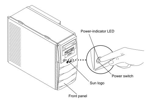
FIGURE 9-3 Workstation Power Switch
