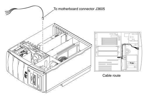
FIGURE 6-11 Removing and Replacing the Logo LED Cable Assembly
