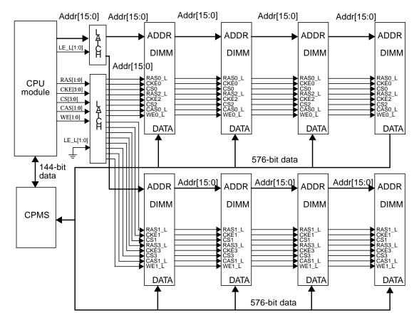
FIGURE C-3 Main Memory Functional Block Diagram
