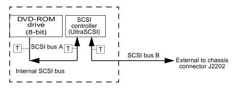
FIGURE C-14 Configuration for the SCSI Bus
