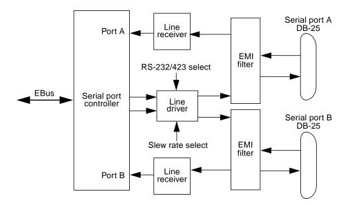
FIGURE C-11 Serial Port Functional Block Diagram
