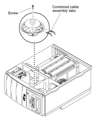
FIGURE 6-15 Removing and Replacing the Speaker Assembly
