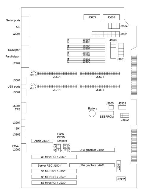
FIGURE C-15 System Motherboard Block Diagram
