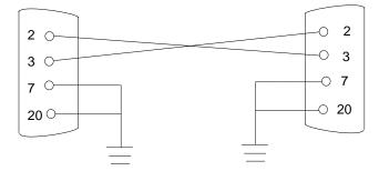
FIGURE 3-1 Setting Up a TIP Connection
