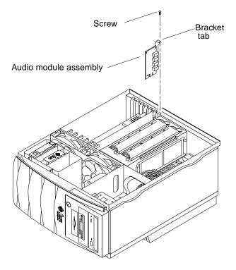
FIGURE 8-18 Removing and Replacing the Audio Module Assembly
