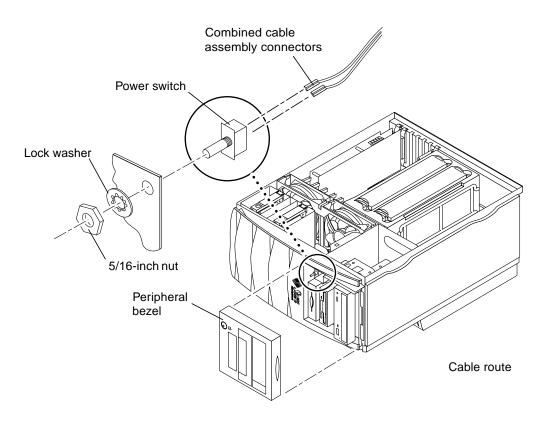
FIGURE 6-5 Removing and Replacing the Power Switch Assembly
