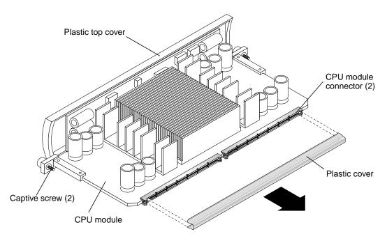
FIGURE 8-8 Removing the Plastic Cover From the CPU Module Connectors
