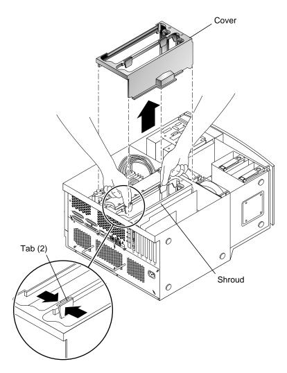
FIGURE 8-6 Removing the Cover for the Shroud
