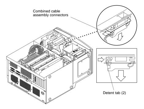
FIGURE 6-12 Removing and Replacing the Interlock Switch Assembly
