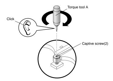
FIGURE 8-14 Torque Tool A Clicks When the Captive Screws Are Correctly Torqued
