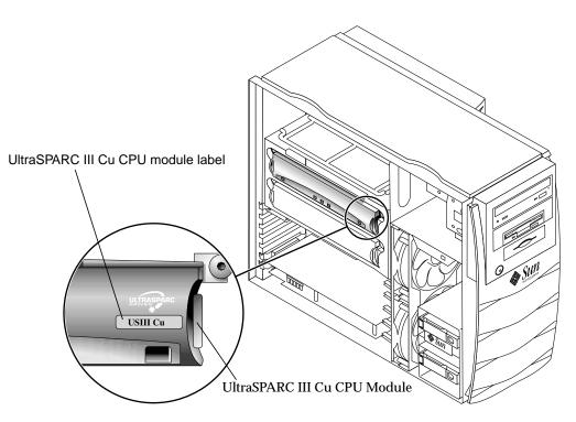
FIGURE 8-1 UltraSPARC III Cu CPU Module and Label
