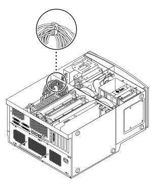
FIGURE 6-1 Power Supply Cable Tie
