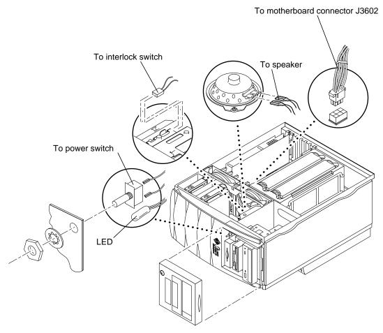
FIGURE 6-10 Removing and Replacing the Combined Cable Assembly
