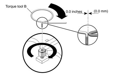
FIGURE 8-11 Adjusting Captive Screws Until the Torque Tool Gap Is 0.0 Inches (0.0 MM.)
