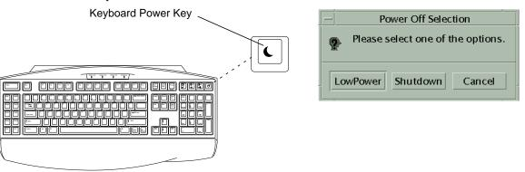
FIGURE 9-4 Sun USB Type-6 Keyboard Power Key and Power Off Selection Dialog Box
