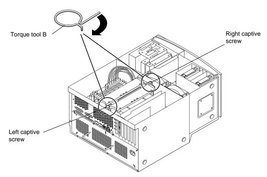
6. Use torque tool B to rotate the right captive screw one turn clockwise (see FIGURE 8-10).
