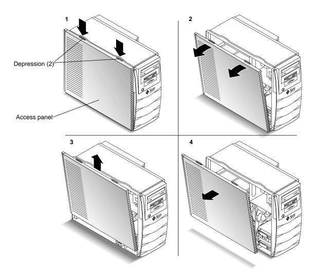
FIGURE 5-3 Removing the Access Panel
