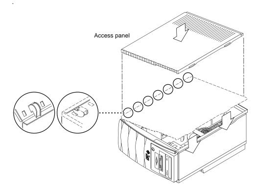
FIGURE 9-1 Replacing the Access Panel
