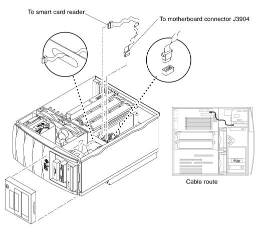
FIGURE 6-9 Removing and Replacing the Smart Card Reader Cable Assembly
