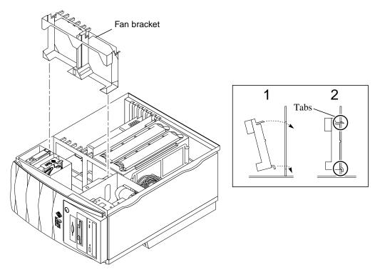
FIGURE 6-14 Removing and Replacing the Fan Bracket
