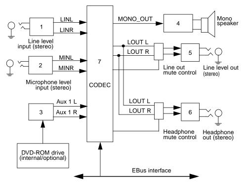
FIGURE C-12 Audio Card Functional Block Diagram
