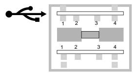
FIGURE B-10 USB Connector Pin Configuration
