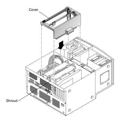
FIGURE 8-12 Installing the Cover for the Shroud
