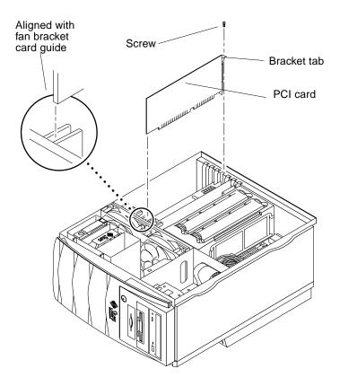
FIGURE 8-15 Removing and Replacing a PCI Card
