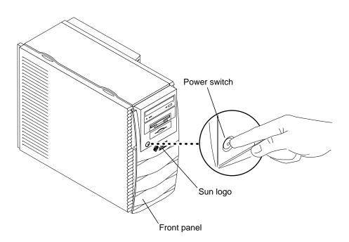
FIGURE 5-1 Workstation Power Switch
