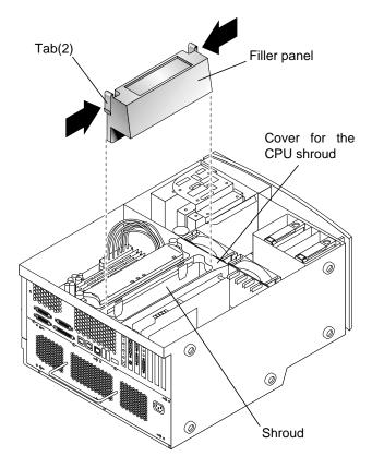
FIGURE 8-4 Removing the Filler Panel
