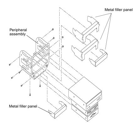
FIGURE 6-19 Removing and Replacing Metal Filler Panels
