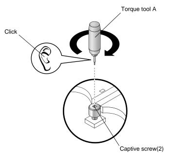
FIGURE 17 Torque Tool A Clicks When the Captive Screws Are Correctly Torqued
