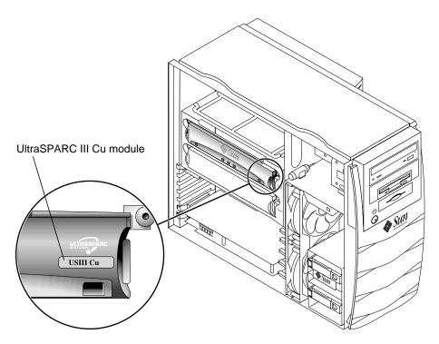
UltraSPARC III Cu CPU Module FIGURE 1
