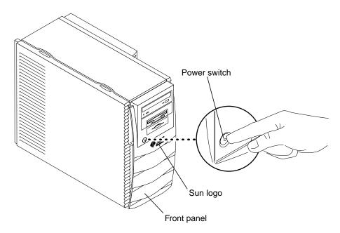
FIGURE 2 Workstation Power Switch
