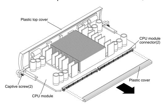
FIGURE 11 Removing the Plastic Cover From the CPU Module Connectors
