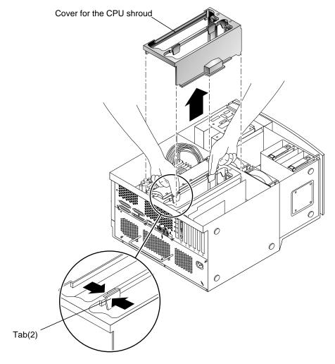
FIGURE 9 Removing the CPU Shroud
