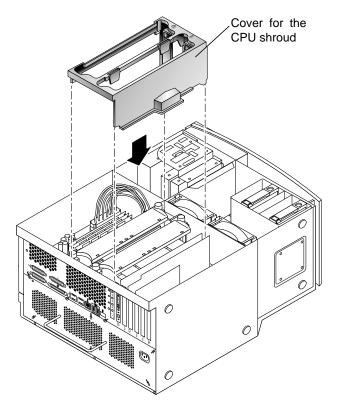
FIGURE 15 Installing the Cover for the Shroud
