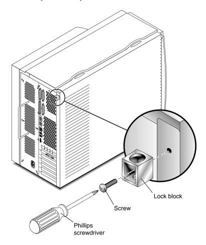
FIGURE 3 Removing the Lock Block
