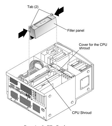
FIGURE 7 Removing the Filler Panel
