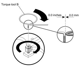
FIGURE 14 Adjusting Torque Tool B Until the Gap is 0.0 Inches (0.0 mm.)
