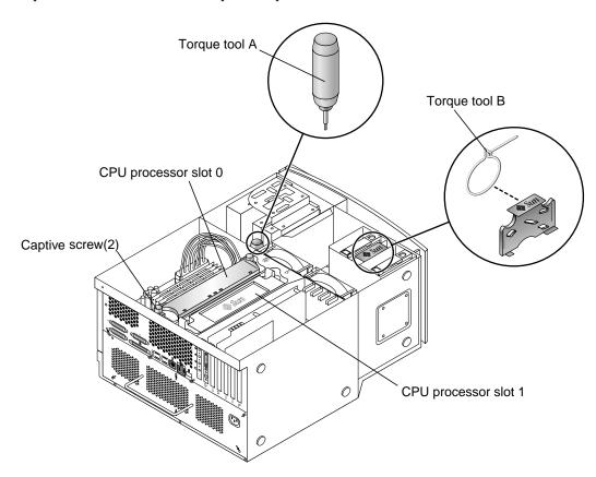
FIGURE 6 Location of CPU Processor Slot 0, Captive Screws, and Torque Tools
