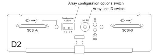
FIGURE 4-1 Sun StorEdge D2 Array Switch Locations
