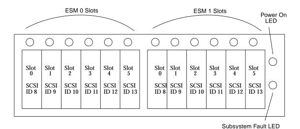
FIGURE 2-4 Sun StorEdge D2 Dual ESM Front View (Split Bus)
