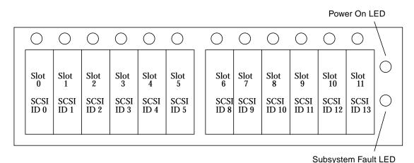
FIGURE 2-3 Sun StorEdge D2 Single ESM Front View (Single Bus)
