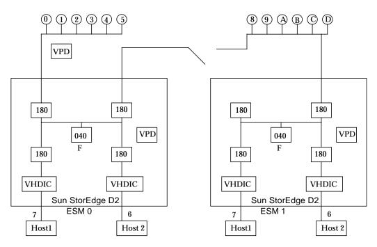
FIGURE 2-2 Dual Sun StorEdge D2 With Split Bus (Logical View)
