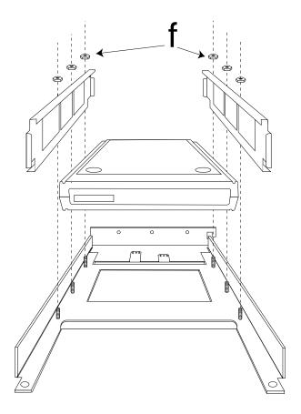
FIGURE 1-3 Securing NTC to NTC Mount
