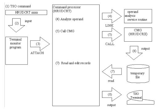
Figure 2.5 Interface Between Command Processor and Operand Analyze Routine
