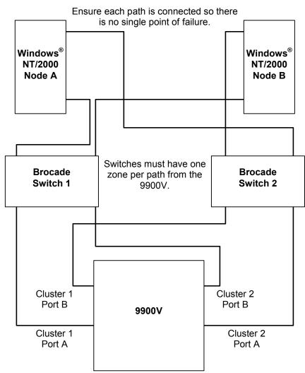
The reason for the isolation between paths is that the cluster resource becomes a virtual device and will cause interaction between the paths when Hitachi Dynamic Link Manager (also HPM) and Clustering are being used together.
