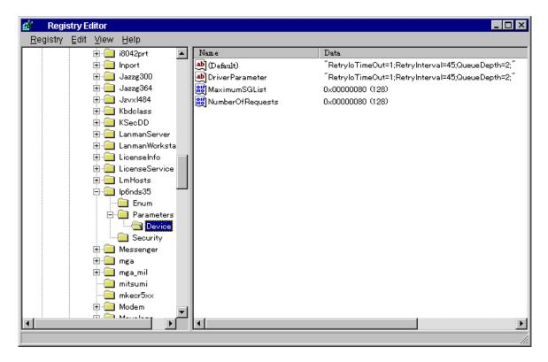
Figure 2.4 Verifying the Queue Depth (Emulex FC adapters shown)
