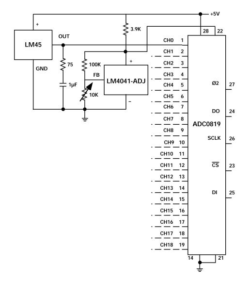
*Figure 5.16. 19-Channel Temperature-to-Digital Converter. Only one LM45 temperature sensor is shown. One LM45 can be connected to each of the ADC0819's 19 inputs.*
