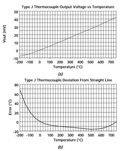
Figure 2.4. (a) Output voltage as a function of temperature for a Type J thermocouple. b) Approximate error in °C vs. a straight line that passes through the curve at 0°C and 750°C
