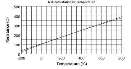
Figure 2.1. RTD Resistance vs. Temperature. The upper curve is a straight line for reference.
