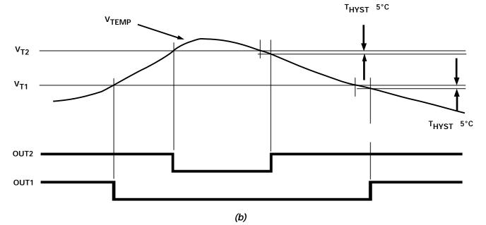
Figure 3.6. (a) LM56 block diagram. (b) Comparator outputs as a function of temperature.
