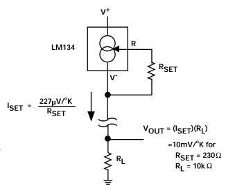
Figure 3.5. LM134 Typical Connection. R<sub>SET</sub> controls the ratio of output current to temperature.
