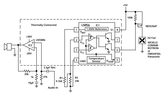
Figure 5.13. This circuit's function is similar to that of the circuit above, except that the sensor, comparator, and voltage reference are integrated within the LM56. In this circuit, the fan turns on at 80°C and off at 75°C.
