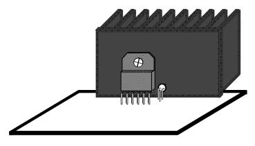
Figure 4.1. TO-220 power amplifier and TO-46 sensor mounted on heat sink. Excellent results can also be obtained by locating the sensor on the circuit board very close to the amplifier IC's leads.
