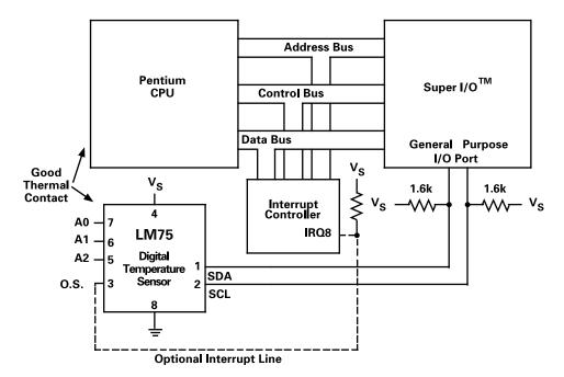
Figure 5.5. Place the LM75 near the microprocessor to monitor the microprocessors temperature in a motherboard application. Temperature data can be read at any time over the two-wire, I<sup>2</sup>C compatible serial interface. Up to 8 LM75s can share the same serial bus if their addresses are set to different values using A0, A1, and A2.
