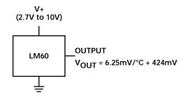
Figure 3.4. LM60 Typical Connection
