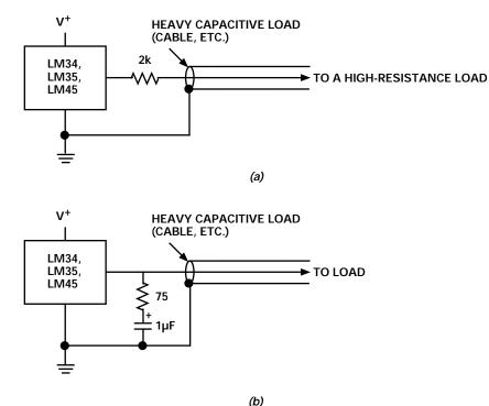
Figure 4.5. Capacitive drive options. The LM34, LM35, and LM45 can drive large external capacitance if isolated from the load capacitance with a resistor as in (a), or compensated with an R-C network as in (b).
