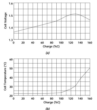
Figure 5.9. Typical NiCd Fast Charging Curves. Note that both cell voltage and cell temperature provide indication of overcharging.
