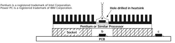
Figure 4.2. Three potential sensor locations for high-performance processor monitoring.
