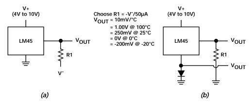
Figure 4.4. Two ways to measure negative temperatures with single-supply sensors. (a) If a negative supply voltage is available, use a pulldown resistor to allow the sensors output to go below ground. (b) Alternatively, bias the "ground" pin using a diode, a voltage reference, or other voltage source. The differential output voltage will be negative for negative temperatures.
