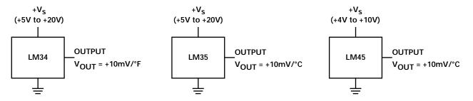
Figure 3.2. LM34, LM35, LM45 Typical Connections. Each IC is essentially a 3-terminal device (supply, ground, and output), although some are available in packages with more pins.
