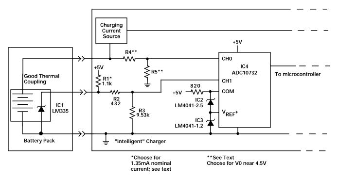
Figure 5.11. Voltage-Output Battery Pack Temperature Sensor
