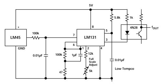
Figure 5.18. Isolated Temperature-to-Frequency Converter
