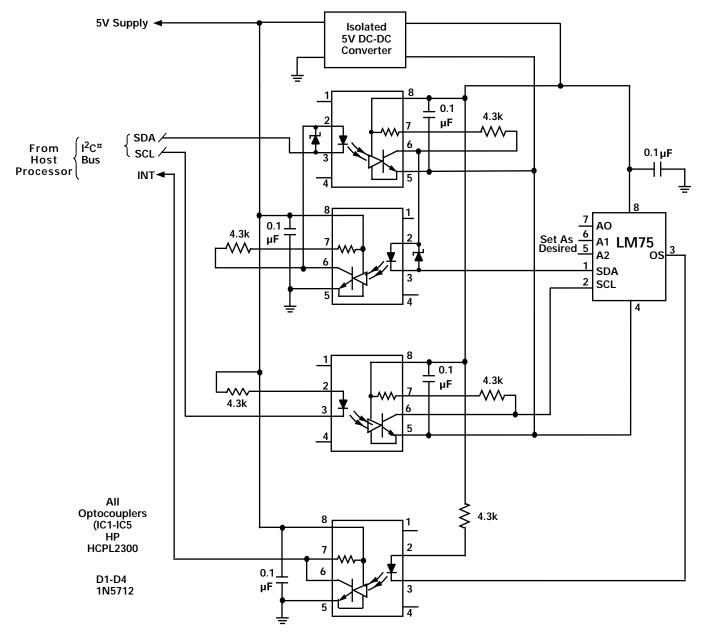
Figure 5.7. Isolated PC-Based Thermometer.
