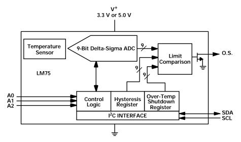
Figure 3.7. LM75 Block Diagram.
