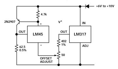
Figure 5.15. 4-20mA Current Transmitter Temperature Sensor
