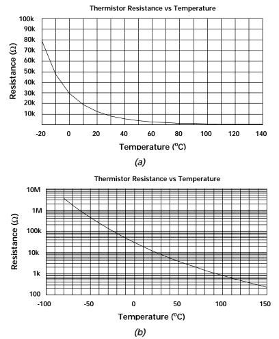
Figure 2.2. Thermistor Resistance vs. Temperature. (a) linear scale. (b) logarithmic scale.
