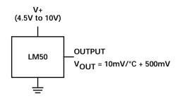
Figure 3.3. LM50 Typical Connection
