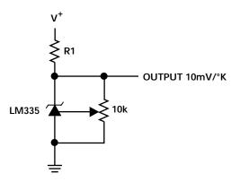
Figure 3.1. Typical Connection for LM135, LM235, and LM335. Adjust the potentiometer for the correct output voltage at a known temperature (for example 2.982V @  $25^{\circ}$ C), to obtain better than  $\pm 1^{\circ}$ C accuracy over the -55°C to +150°C temperature range.
