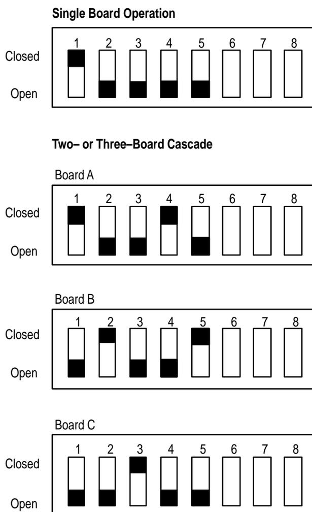
**Figure 2. Switch Positions**
