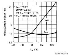
FIGURE 2. Delay vs Temperature
