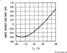
FIGURE 3. Offset Temperature Coefficient
