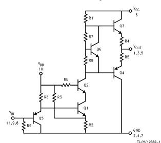
FIGURE 1. Simplified Schematic Diagram (One Channel)
