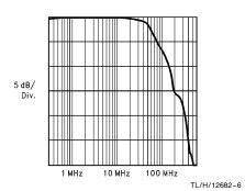
FIGURE 5. Large Signal Frequency Response
