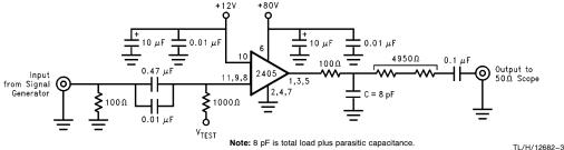
Note: Adjust Vtest for +2.6V DC at LM2405 input pins. See
