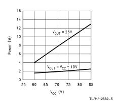
FIGURE 4. Power Dissipation vs V<sub>CC</sub>
