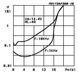
Figure 15: Distortion vs. Output Power
