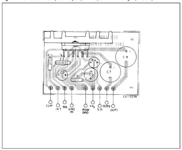
Figure 3: BRIDGE Test and Application Circuit
