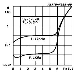
Figure 13: Distortion vs Output Power (Stereo)
