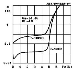
Figure 12: Distortion vs Output Power (Stereo)
