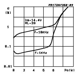
Figure 14: Distortion vs Output Power (Bridge)
