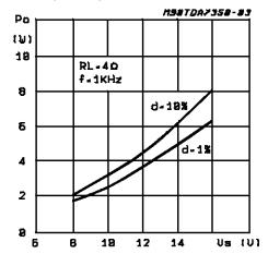
Figure 7: Output Power vs. Supply Voltage (Stereo)
