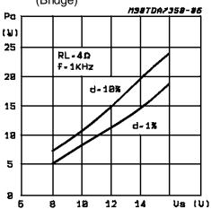
**Figure 9:** Output Power vs. Supply Voltage (Bridge)
