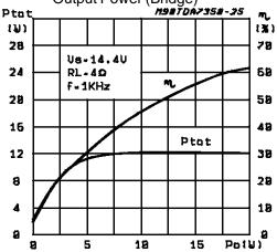
**Figure 22:** Power Dissipation & Efficiency vs. Output Power (Bridge)
