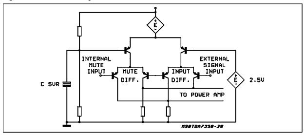
Figure 25: Turn-on Delay Circuit
