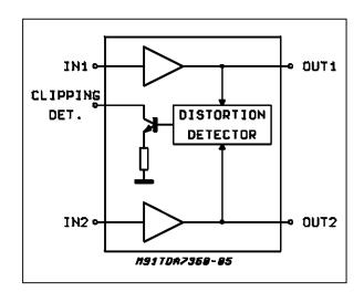
out. (pin2) when a certain distortion level is reached at each output. This particular function allows compression facility whenever the amplifier is overdriven, so obtaining high quality sound at all listening levels.
