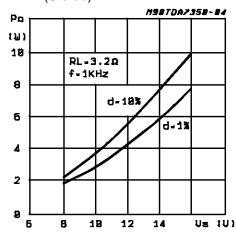
**Figure 8:** Output Power vs. Supply Voltage (Bridge)
